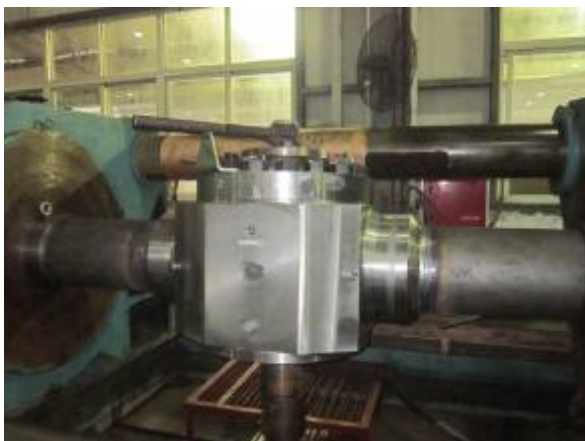
DBB water seal testing (No leakage)
