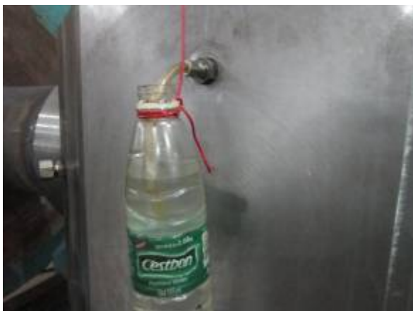
Air seal testing (No leakage)
