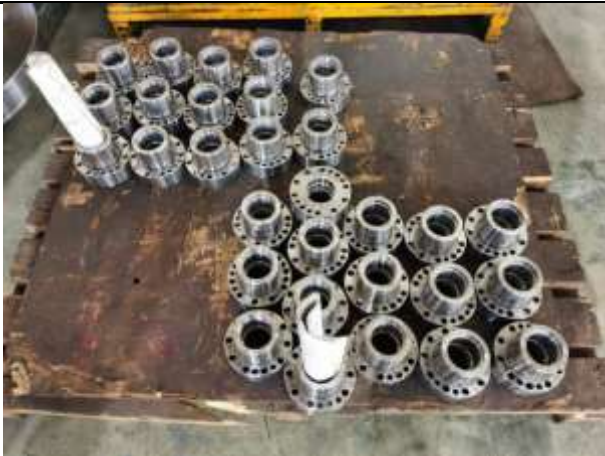
Seal sleeve machined (SSO-305-2022)
